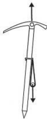
Strength test of the attachment device
